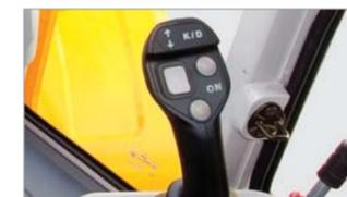
**FNR Switch on Joystick Control Lever**
