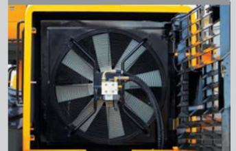
The minimum fuel consumption and low noise is realized by applying hydraulic cooling fan that senses coolant temperature, intake air temperature, transmission oil temperature and hydraulic oil temperature.
