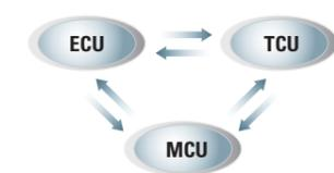
Engine control Unit(ECU), Transmission control Unit(TCU) and Machine control Unit(MCU) realize the optimal performance through the mutual CAN communications.
