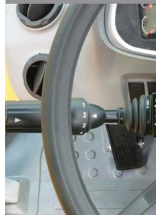
A single lever on the left side of the steering column gives the operator fast, easy control of speed and direction. Push the lever forward to go forward, pull it back for reverse. Travelling is automatically changed from 1st stage to given stage according to travel speed and tractive effort. The operator can select two kinds of automatic modes (1st ↔ 4th, 2nd ↔ 4th). These exclusive features contribute to a step-up in productivity and reduction of operator's fatigue.
