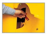
Transmission oil port The transmission oil change port is also located for with open accessibility and comes with an anti-vandalism lock for your machine protection.
