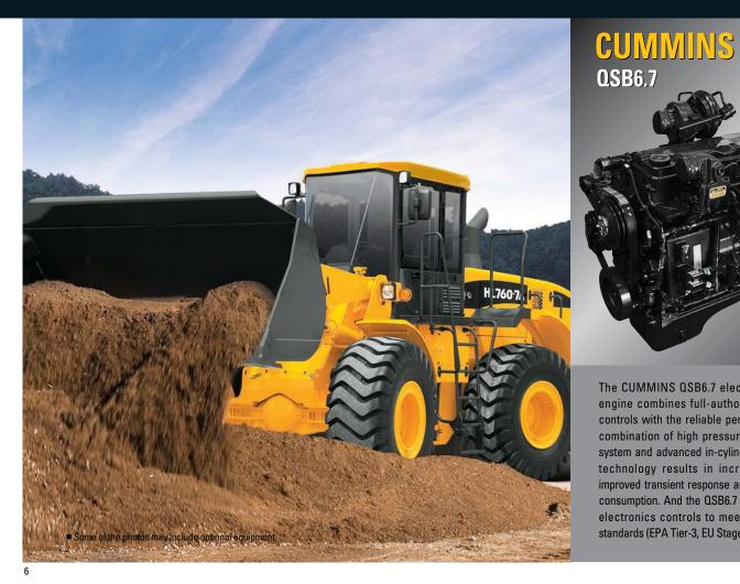
The CUMMINS QSB6.7 electronic control engine combines full-authority electronic controls with the reliable performance. The combination of high pressure common rail system and advanced in-cylinder combustion technology results in increased power, improved transient response and reduced fuel consumption. And the QSB6.7 used advanced electronics controls to meet the emission standards (EPA Tier-3, EU StageIII-A )
