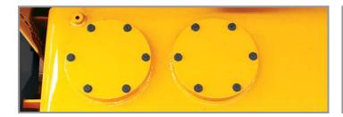
Hydraulic tank The hydraulic tank is located behind the cab to increase the accessibility of hydraulic hoses and pipings.
