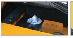
**Battery master switch** A master switch disconnects the battery power to protect the electrical system from excessive electrical drainage.
