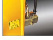
**Remote type drain port** It is now easier to change your engine oil, coolant and hydraulic oil with the remote drain port.
